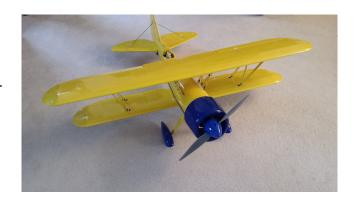
This version was designed for a 40-60 nitro engine, but I chose to convert it to electric using an E-flite Power 60, Castle Creation Talon 90 (one of the few ESC's with a built in BEC providing 9amps continuous current) and a Turnigy 5000mAh 6S 65C A-Spec G2 LiPo. (Look it up.) This combination should provide plenty power for 3D maneuvers and a virtually unlimited vertical climb rate.
