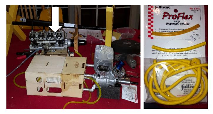
The Sullivan tubing is a bit on the expensive side so I am using it only for internal tank plumbing. But if it lives up to its advertising the tubing will be much more cost effective and less labor intensive than having to remove and replumb every gas tank prior to the start of each new season.
